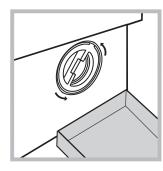
2. position a container so that it will collect the water which flows out (approximately 1.5 l) (see figure);
